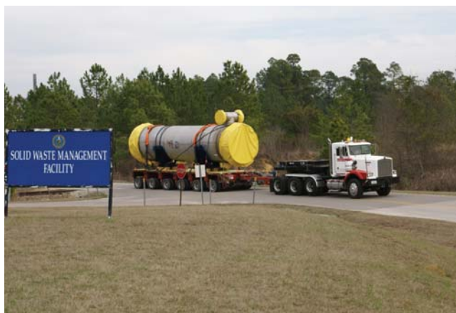
Heat Exchangers Transported for Disposal
