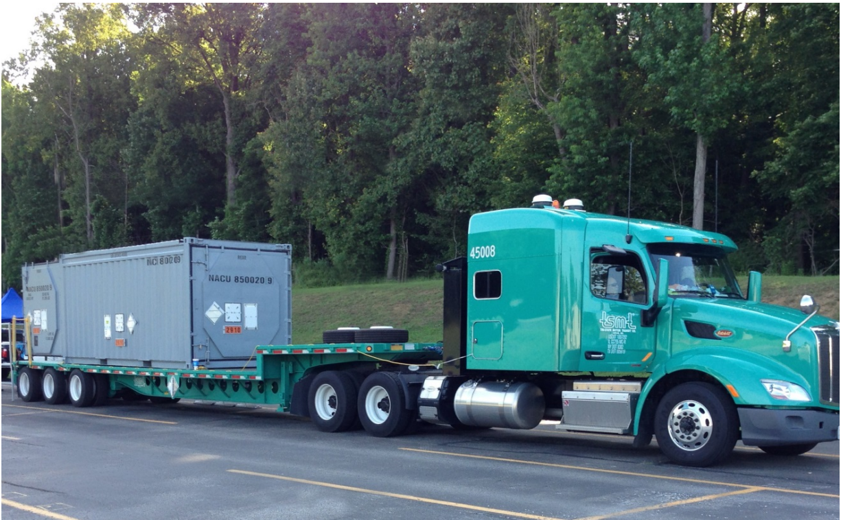
Figure 1. Transport Truck with ISO Container in which the NAC-LWT Cask is Carried
