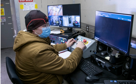
Remote operation allows for the characterization of a transuranic waste drum using the RTR unit.
