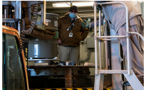
A transuranic waste drum is loaded into the RTR unit for characterization.
