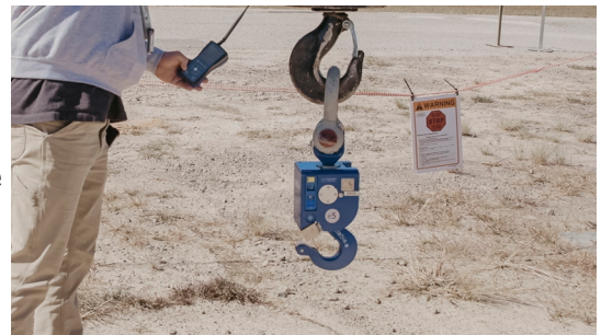
The remote release hook allows riggers to place low-level radioactive waste in a slit trench with less potential for contamination.
