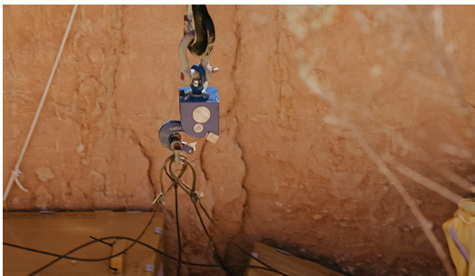
The remote release hook disengaging from rigging after lowering low-level waste into a slit trench.
