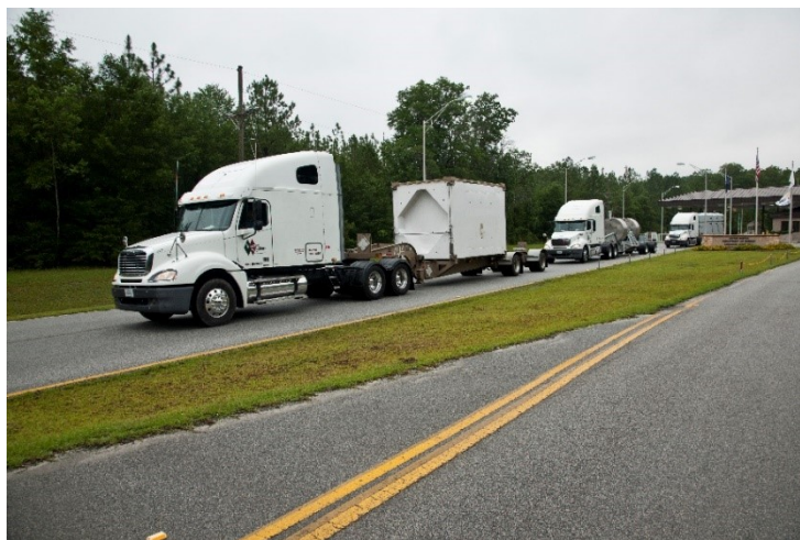
SRS made DOE Complex history in 2012, when it made three TRU waste shipments on the same day, using three different shipping containers. The three trucks transporting TRU waste (from left) used TRUPACT-III, RH-72-B and TRUPACT-II containers.
